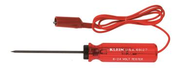
This device checks live 6-24V, AC or DC circuits. Tests for shorts in automotive and truck electrical systems, motor field coils, radio and low-voltage circuits, ground circuit of all lamps, wiring, fuses, etc. Pointed 3-3/4" (95 mm) probe makes checking easier.
