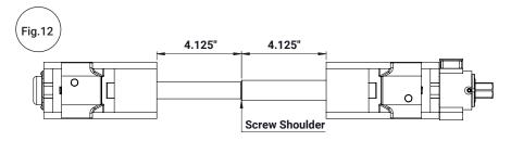
Reset Timing - Rotate Nuts until the 4.125" Spacing above is achieved
