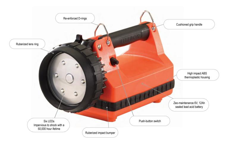
6 LEDs wide pattern parabolic reflectors produce a smooth flood pattern; optimized electronics provide regulated intensity
