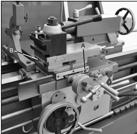
Figure 25 – Gib adjustments, slide and rest
