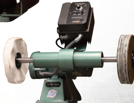
The 1001 can run up to 12" diameter wheels up to 2" wide. Dust scoops can be added as an optional accessory.
