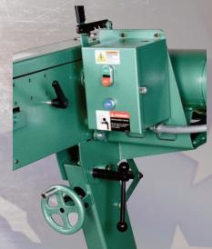
Optional magnetic starter and easy to adjust elevation controls
