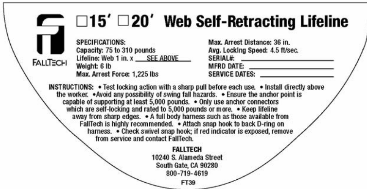
Fig. 10.2 Product label for FallTech Web SRL's 7270WR, 7271WR and 7270KV (Located on front housing)
